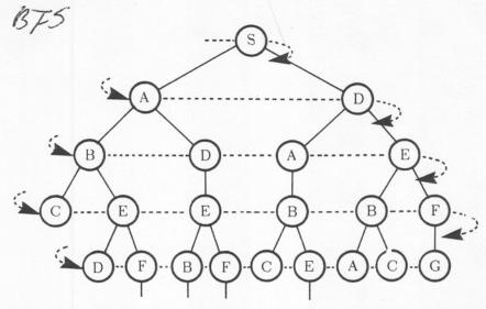
Figure 4-7. An example of breadth-first search. Downward motion proceeds level by level until the goal is reached.
