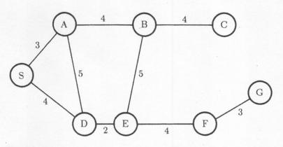
Figure 4-2. A basic search problem. A path is to be found from the start node, S, to the goal node, G. Search procedures explore nets like these, learning about connections and distances as they go.
